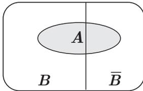
$$P(A) = P(A \cap B) + P(A \cap \bar{B}) = \\ = P(B) \times P(A | B) + P(\bar{B}) \times P(A | \bar{B})$$
